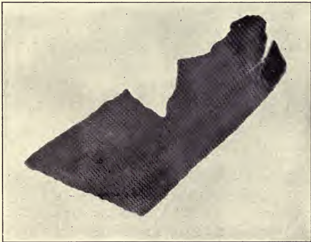
FIG. 411.—The Radio-active Effect of a Portion of a Gas Mantle on a Photographic Plate.
